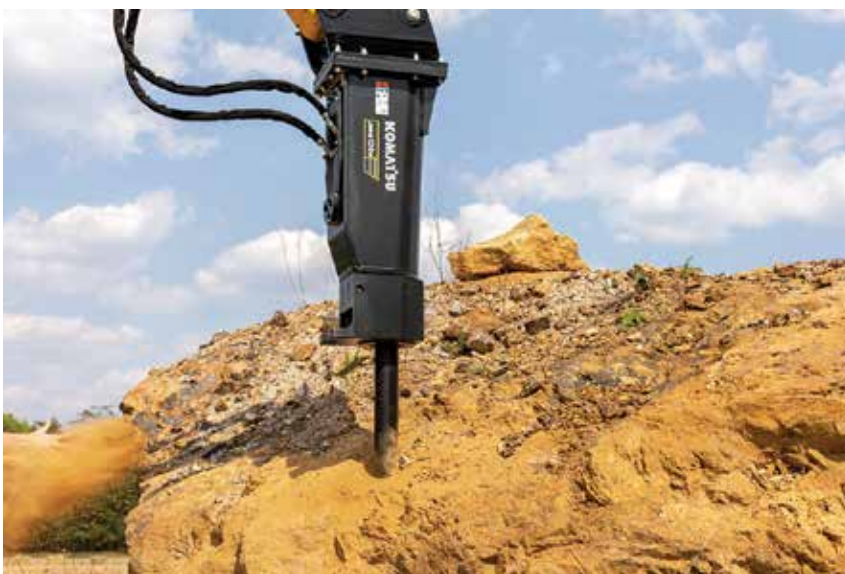
Komatsu built in several features and benefits to protect the breaker, carrier and operator – including an accumulator that recycles high-pressure oil internally and reduces surges back to the carrier. This allows the creation of more energy with lower flow and reduces hydraulic pressure spikes. The breakers also have blank fire protection and automatic pressure regulation.
