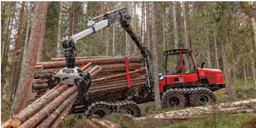
The 845 forwarder is Komatsu's new entry into the 12-metric-ton-capacity class. It offers the latest version of Komatsu's patented, rugged FlexGate headboard, which "flexes" if hit by the crane or a log (also standard on the 895 and optional on the 855).
