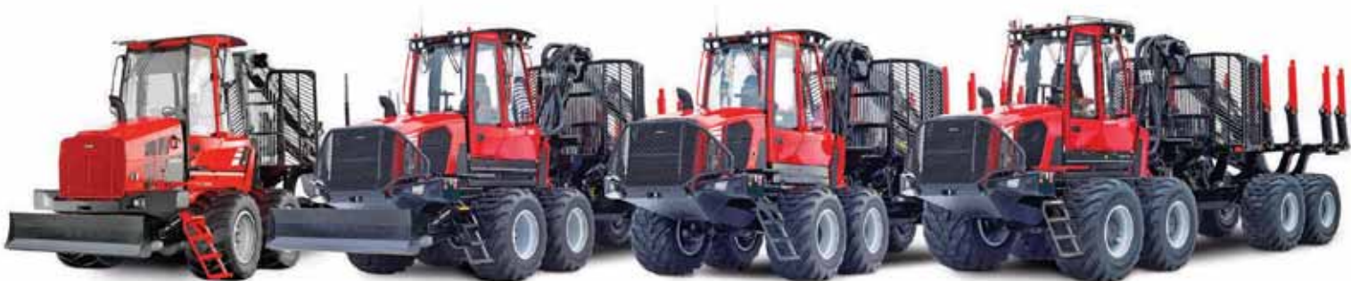
The new Komatsu 845, 855, 875 and 895 Tier 4 Final forwarders have rated payload capacities of 12, 14, 16 and 20 metric tons, respectively.
