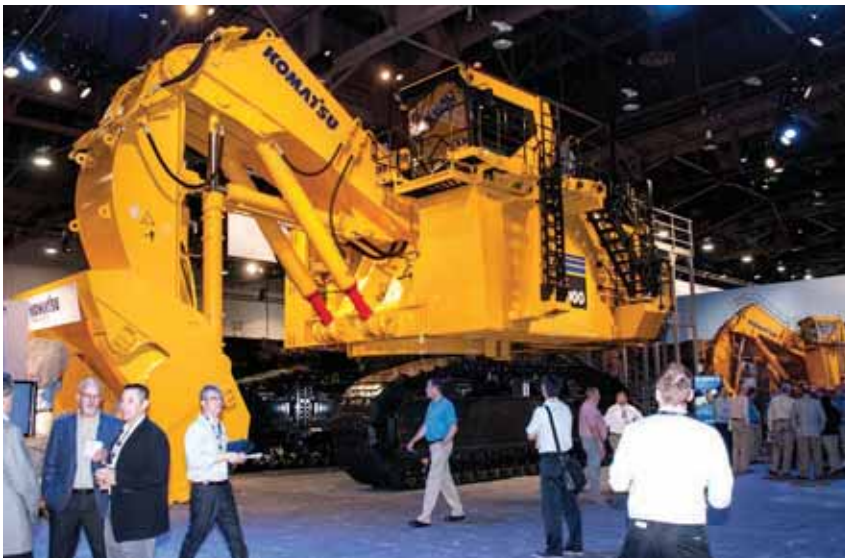
Attendees check out the new Komatsu PC4000-11 at MINExpo 2016. It features a Tier 4 Final 1,875-horsepower engine and can be configured as a shovel or backhoe.
