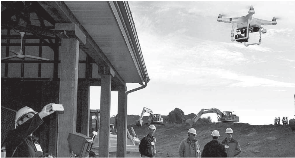
Drones/UAVs can be controlled from the ground with computers, smart phones and tablets and provide a birds-eye view of a site on the device. Users control the flight path, and cameras can take pictures for documentation and other purposes. Aerial photo courtesy of Cadre Solutions Group.
