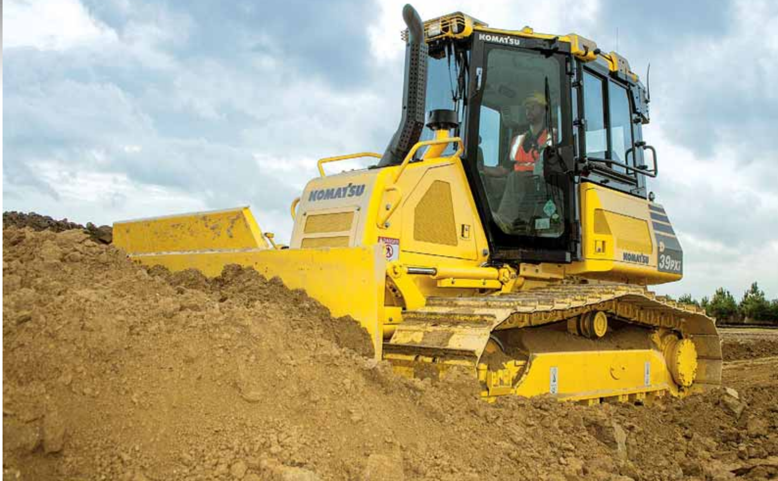
Komatsu's intelligent Machine Control lineup now features four models, including the new D39PXi-23. All have integrated technology that provides automated grading from rough-cut to finish grading.
