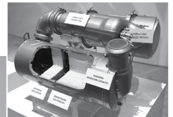
Komatsu displayed the technology behind its Tier 4 Final engines, including the selective catalytic reduction components (inset) that reduce emissions to near zero.
