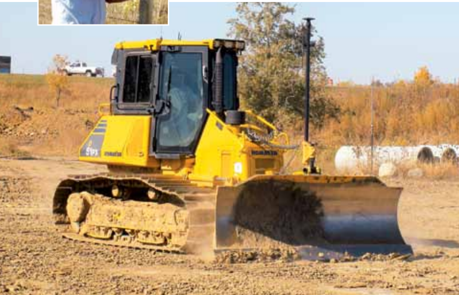
Brad Schoenfelder sets up a Topcon 3D-MC 2 base unit used to set grade via GPS with a Komatsu D51 dozer. Schoenfelder Construction shaved months off a site-work project with the Topcon/Komatsu combination.
