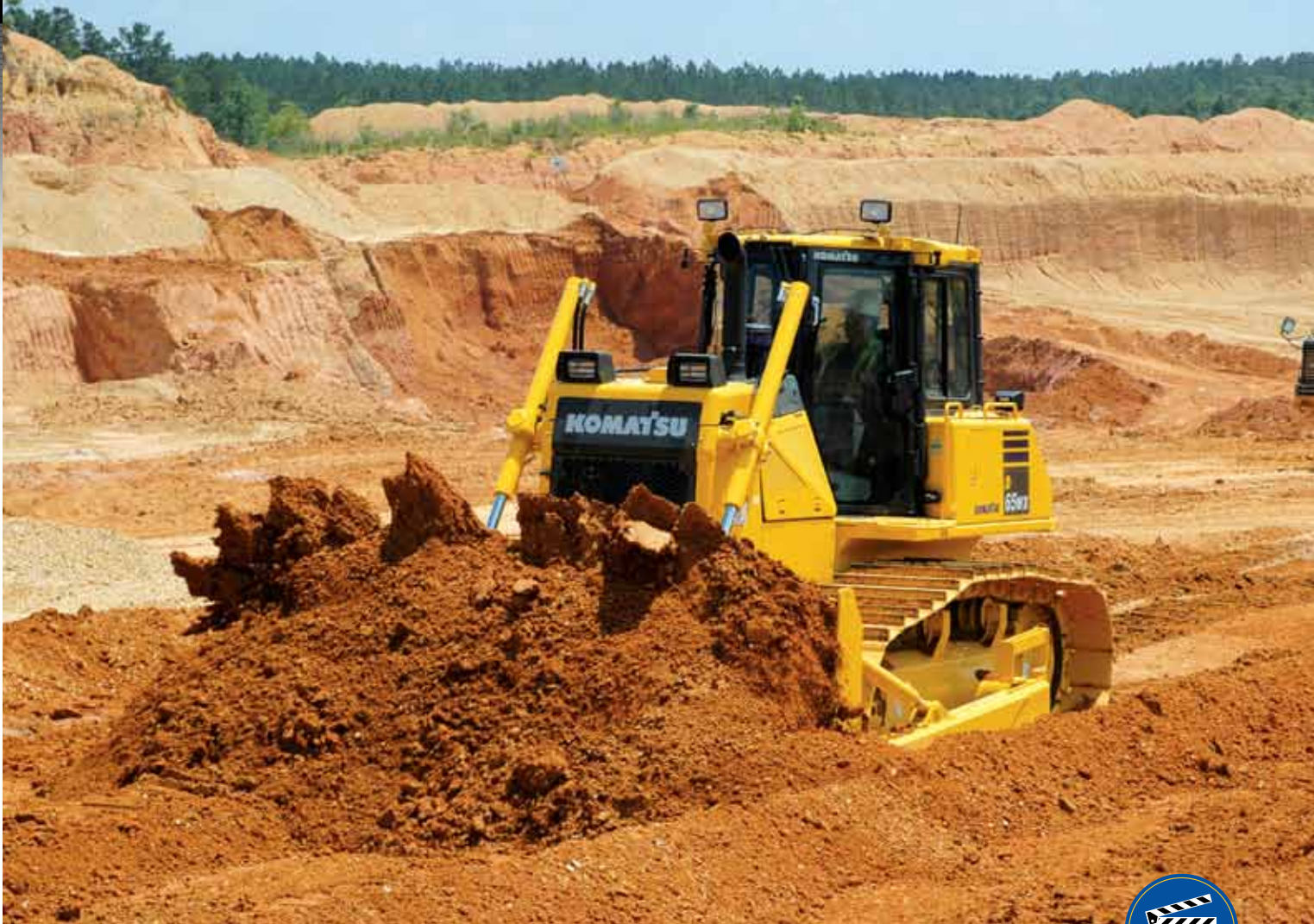
Last year, Komatsu introduced new excavators, articulated dump trucks and dozers, including this D65-17, that meet Tier 4 Interim standards. Data show they're more fuel-efficient and productive, with lower emissions than their Tier 3 predecessors.
