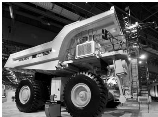
A Komatsu 860E-1KT has 2,700 horsepower for moving mass amounts of material faster.
