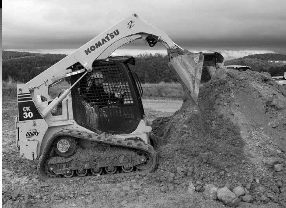
Utility machines, such as the CK30 compact track loader, were required to meet Tier 4 emission standards in 2008. Tier 4 is on the horizon for 175 horsepower and up machines in 2011 and 75 to 175 horsepower must be Tier 4 in 2012.
