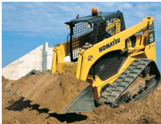
Komatsu's compact track loaders are equipped with a five-roller track system to keep track deflection and damage to a minimum. Triple-flange rollers and track guides allow for use on slopes without detracking.
