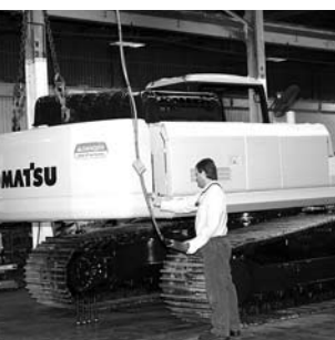
Using an overhead crane, a worker installs the counterweight on a PC300LC-7 at the Chattanooga plant.
