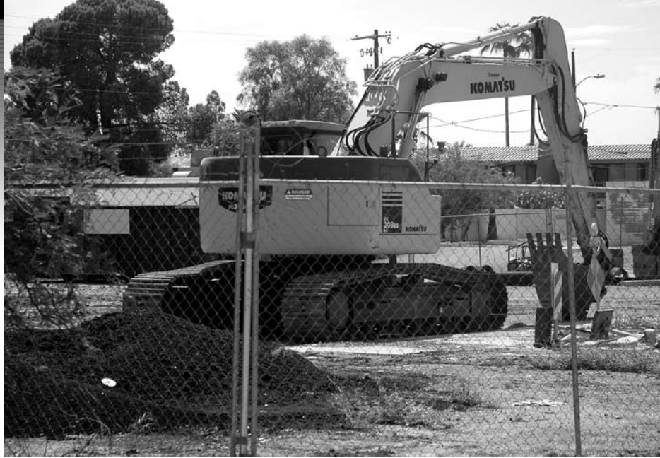
When not in use, equipment should be parked in a fenced-in area that contains barbed or razor wire, if possible. Fencing should have a heavy-duty gate with a case-hardened chain and high-security padlock.
