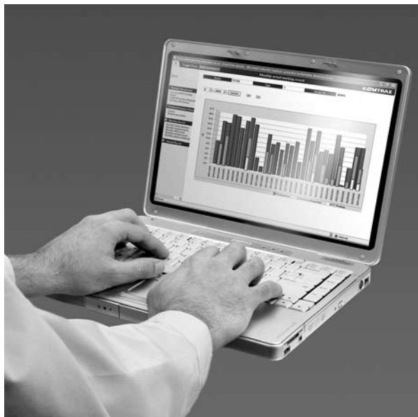
GPS systems, such as Komatsu's Komtrax wireless monitoring system, allow users to monitor and track equipment continuously. If criminals know the machines have GPS tracking devices, they are less likely to take them.
