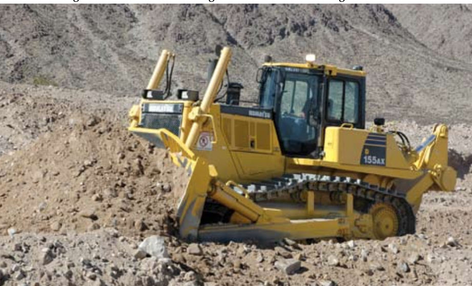
The D155AX-6 is the first construction-class machine to get the K-Bogie undercarriage, the larger and sturdier undercarriage used on Komatsu mining dozers.
