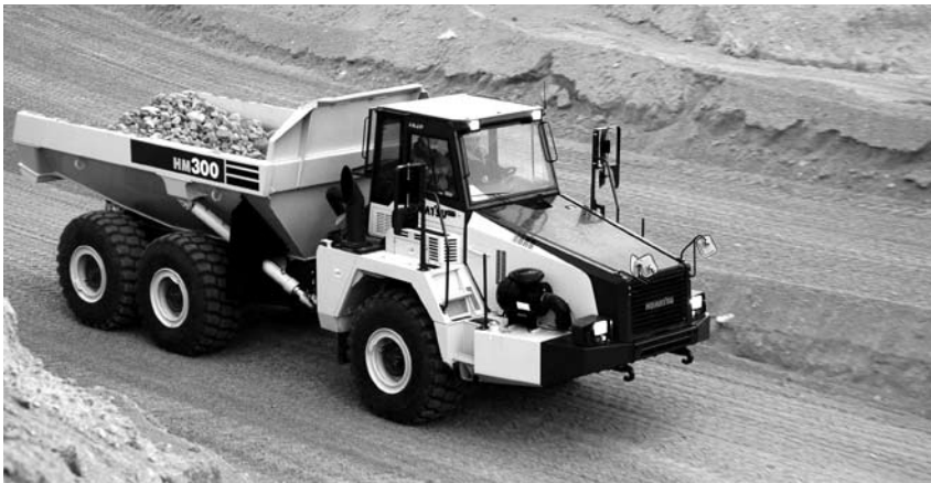
Among a host of new Komatsu products this year is the HM300-2 articulated truck. The unit features a significantly reinforced front bumper and engine guard as well as a new transmission guard. The new ecot3 engine boosts horsepower and low-end torque, which helps make the new truck about 11 percent more productive than its predecessor.
